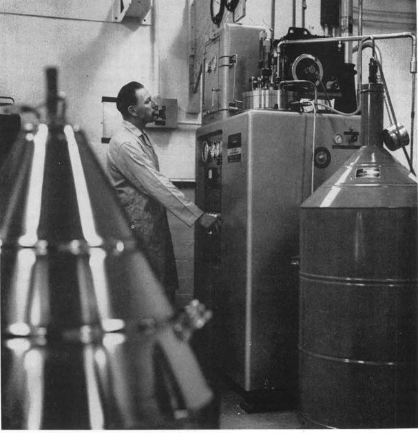
THIS ADL-COLLINS helium refrigerator, installed in Bldg. 855 last month, is used to achieve a nearperfect vacuum for materials testing. Ray Drury
